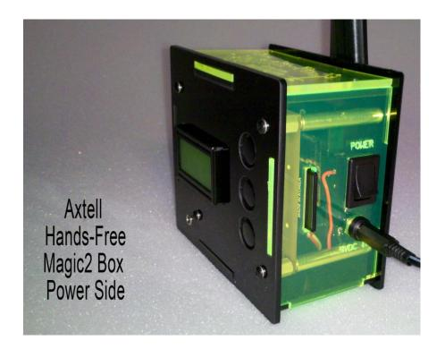
Use the provided A/C adapter to power your box. This should be plugged into the jack located directly underneath the on/off switch.
